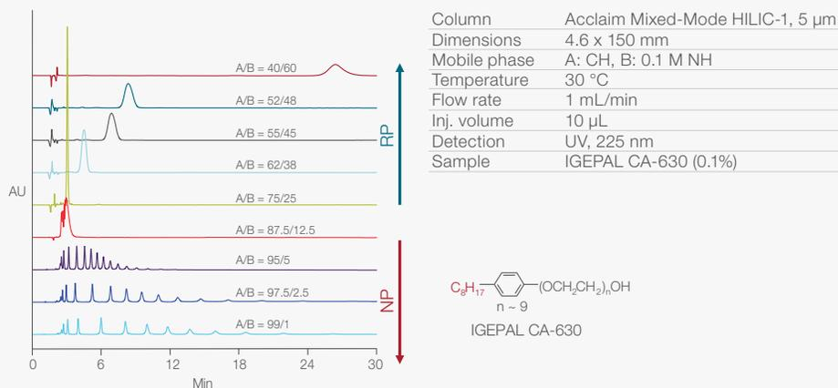
Figure 3. Reversed-phase and normal phase modes on a single column.
