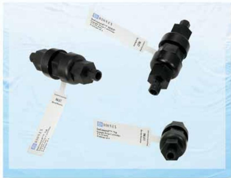
*The InGuard™ line of sample pretreatment cartridges is designed to remove matrix interferences such as cations (including transition metals), anions, or hydrophobic substances that are encountered in many ion chromatography (IC) applications. The InGuard cartridge is installed in-line between the autosampler and the IC injection valve, facilitating immediate, automated sample pre-treatment.*
