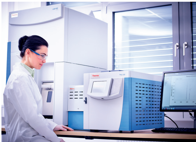
Figure 1. The Thermo Scientific iCAP RQ ICP-MS connected to a Thermo Scientific TRACE 1310 GC with the dedicated Thermo Scientific GCI 100 Interface.
