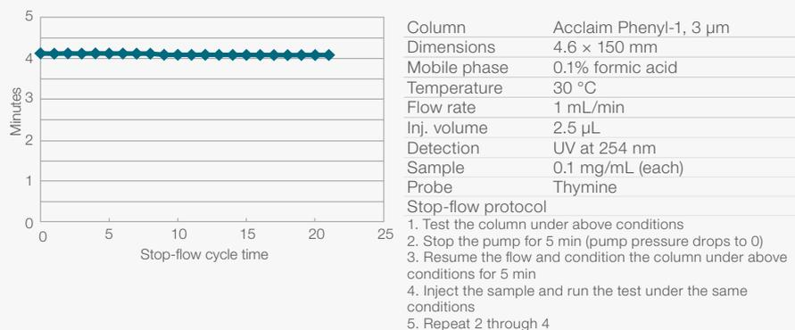
Figure 5. Compatibility with aqueous conditions
