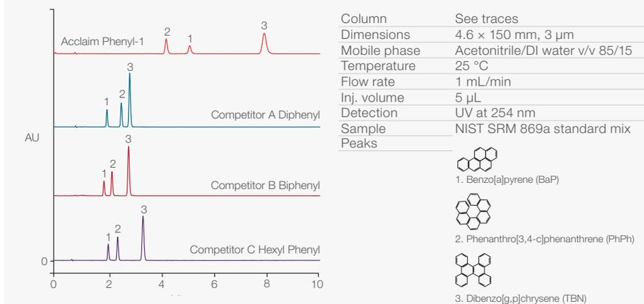
Figure 4. PAH selectivity comparison—separation of NIST SRM 869a
