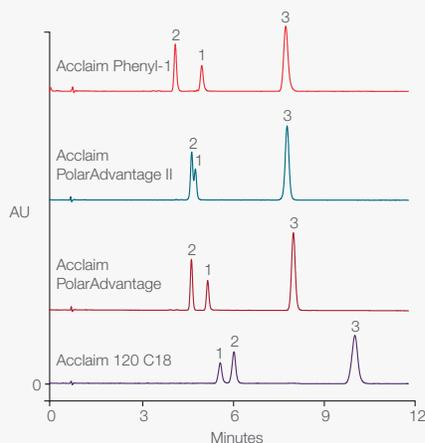
Figure 3. PAH selectivity comparison—separation of NIST SRM 869a
