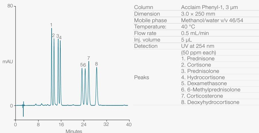
Figure 6. Separation of glucocorticosteroids
