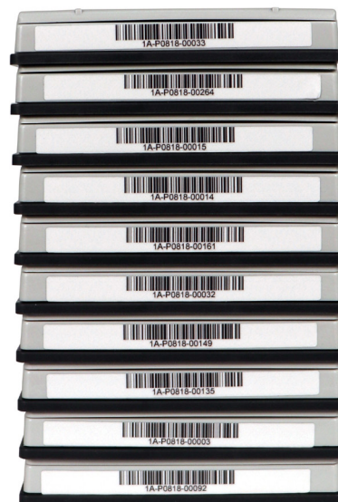
Figure 3. Side view of barcoding on the VeriSpray 24-sample plate.
