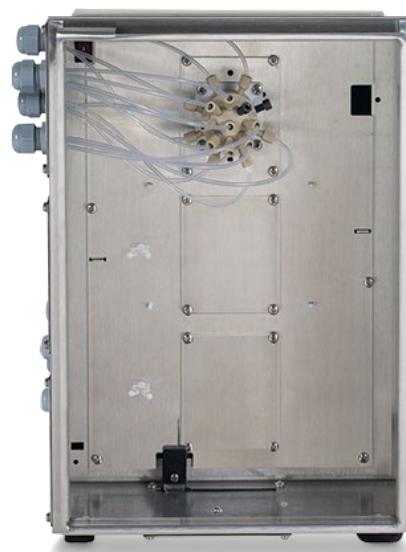
Figure 2. SS module setup with one multiposition valve, door open; up to three valves can be installed
