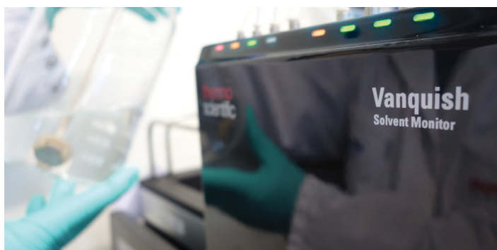
Figure 2. The Vanquish Solvent Monitor provides live feedback as to the fill levels of each solvent channel as well as a waste container ensuring the completion of running sequences
