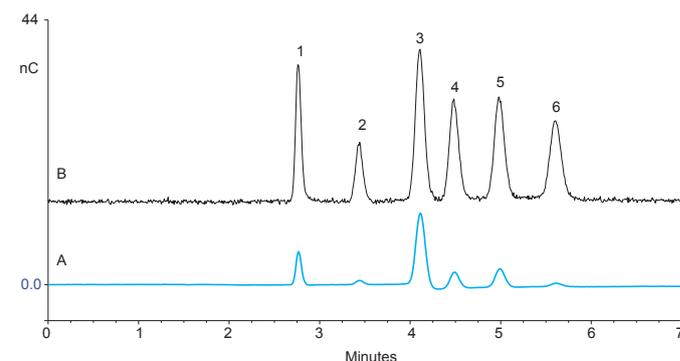
Figure 6. Separation of selected carbohydrates on the Dionex CarboPac SA10 column, (A) Method 2 without postcolumn addition of NaOH and (B) Method 3 with postcolumn addition of 200 mM NaOH at 0.4 mL/min.
