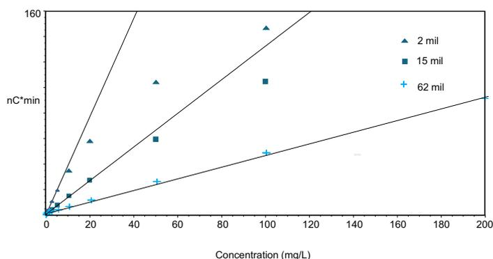
**Figure 4. Calibration data for glucose on 2, 15, and 62 mil gaskets in the concentration range of 0.05–200 mg/L using Method 1.**
