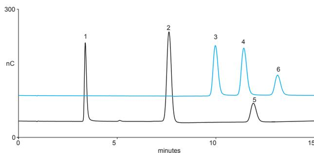
Figure 3. Separation of fucose, glucosamine, glucose, xylose, sucrose, and fructose, each at 10 mg/L, on the Dionex CarboPac PA20 column using Method 1.
