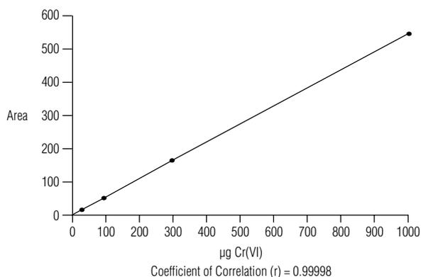
Figure 4. Area response for colorimetric chromium detection.
