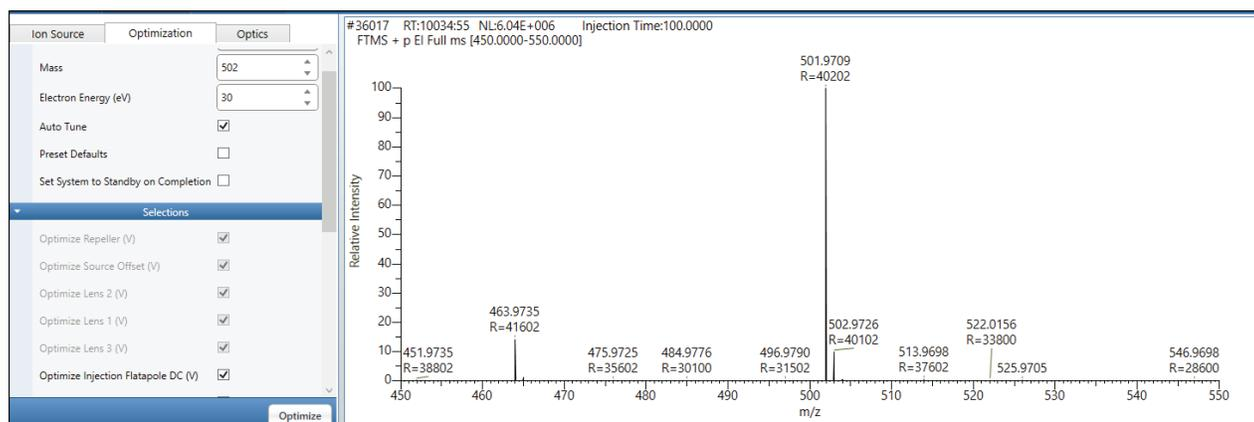
Figure 1. Orbitrap Exploris GC tune VeV window. The eV and tune mass can be selected by the user prior to tuning that takes < 1 minute.
