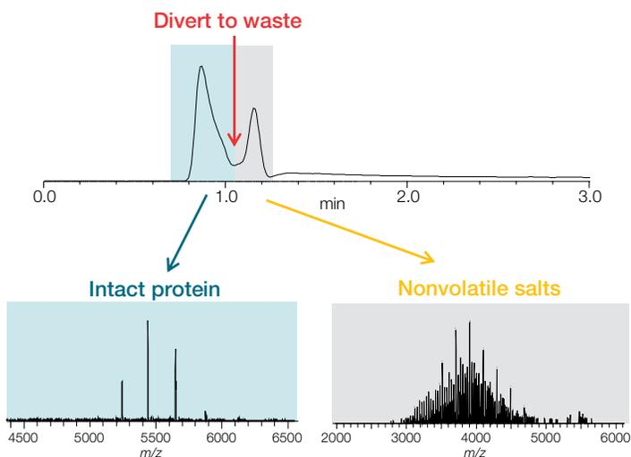
Figure 1. A typical chromatogram from the OBE method
