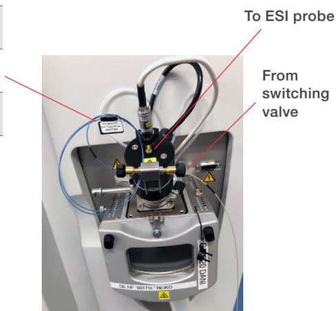
A 75  $\mu\text{m}$  × 650 mm (P/N 6041.5775) “resistor” tubing is fitted between the ESI probe and ground to reduce the spray current and make it possible to utilize mobile phases with high ionic strength
