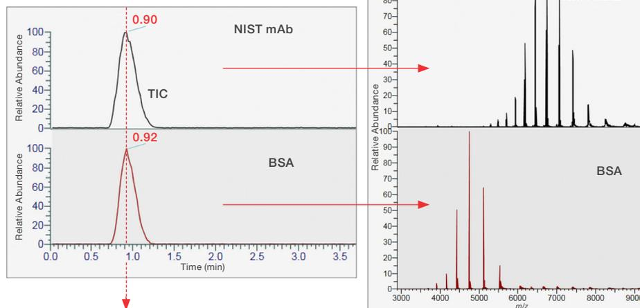
As the proteins used here are above the exclusion limit of the resin (approximately 6 kDa), all proteins elute from the column in the void volume which allows for the development of a single LC-MS method regardless of the size of the biomolecule. Elution time for an individual column remains constant.
