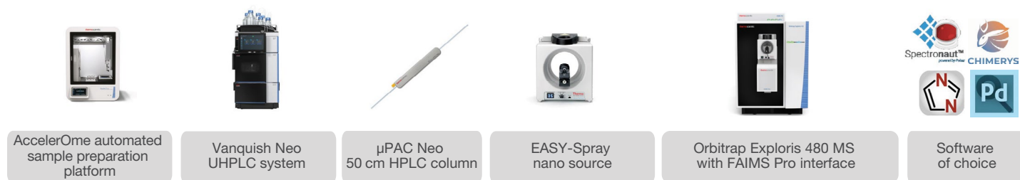
Figure 1. Graphical schematic of the Velocity DIA workflow for label-free quantitation on the Orbitrap Exploris 480 MS together with the optional AccelerOme automated sample preparation platform
