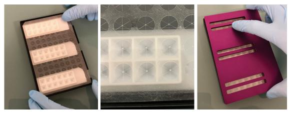
4. Position the holder in the autosampler carousel of the Vanquish Neo UHPLC system such that the "A1" label is in the top left-hand corner.
