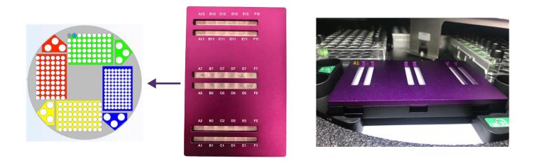
5. To enable the sampler to recognize the holder for sample injection, set the plate type to "WellPlate96" manually on the SII e-panel in the MS controlling PC.
