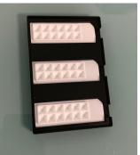
2. Remove the bottom protective film (on the side with the adhesive) of the sealing tape (Thermo Fisher Scientific, P/N 60180-M146/M176). Position the sealing tape over the funnels and peel off the upper protective film.
