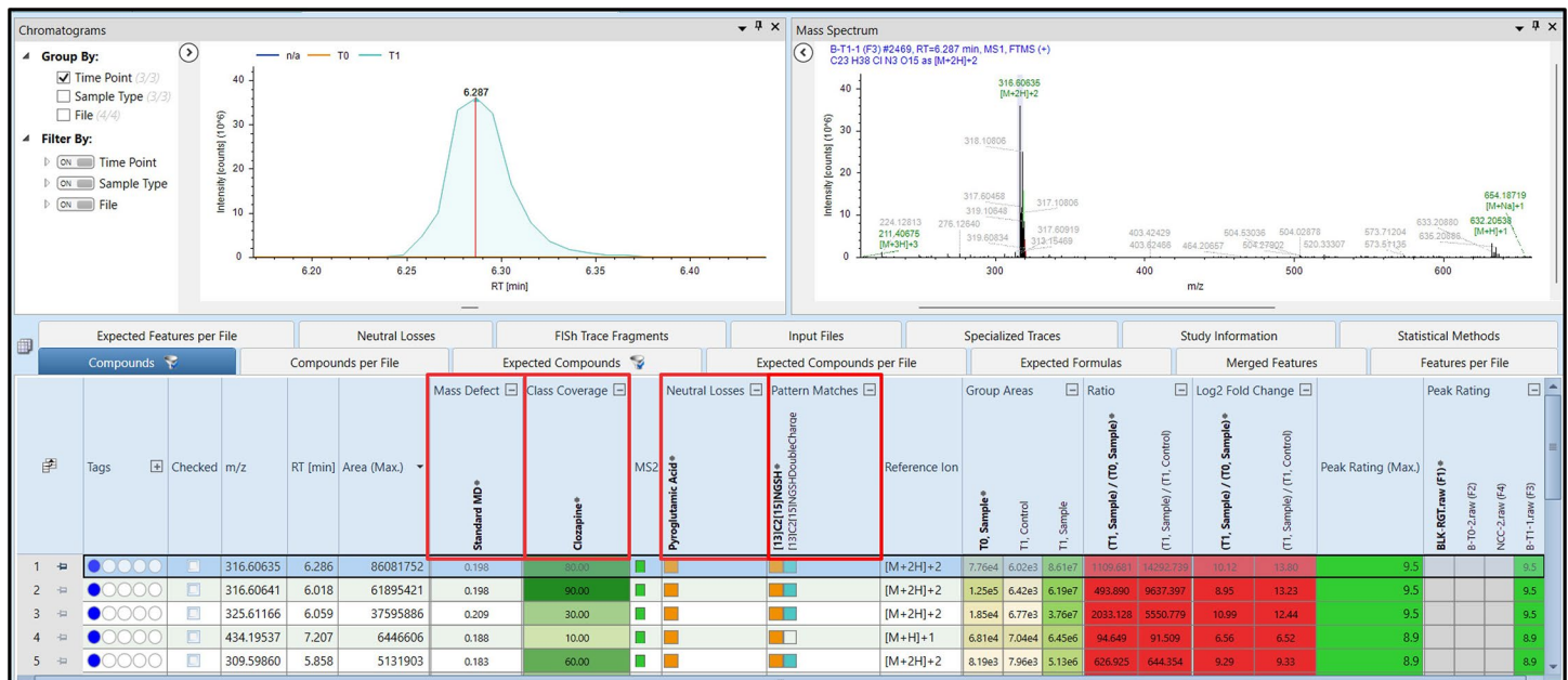
Figure 6. Results view of the Compounds table. The Compounds table organizes information with columns pertinent to the analysis such as Mass Defect, Class Coverage, Neutral Losses, and Pattern Matches (highlighted in red), and it is interactive with Chromatograms and Mass Spectrum views.
