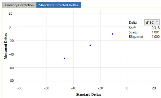
Figure 4. Qtegra ISDS Software data evaluation of measured isotope values vs. known isotope values of a CSIA standard
