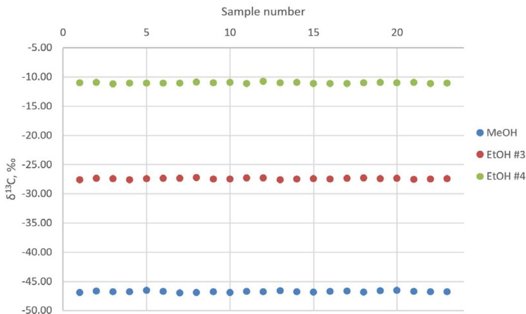
Figure 5. Isotope data acquired in different sequences for the MeOH and EtOH certified standards; 150 ng/μL (150 ppm) in H<sub>2</sub>O using an SHS injection option
