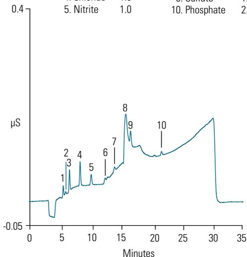
**Figure 8. A large-loop direct injection of a 1:100,000 diluted Dionex Seven Anion II Standard onto a capillary Dionex IonPac AS19 column set. A) 2 mm microbore and B) 0.4 mm capillary columns.**
