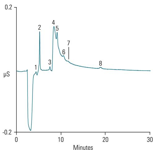
**Figure 9. Trace anions in a water blank injection determined by concentrating 200  $\mu\text{L}$  on a Dionex IonSwift MAC-100 concentrator column.**
