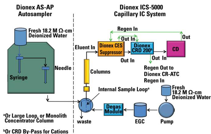
Figure 1. Flow diagram for the Dionex ICS-5000 capillary IC system.
