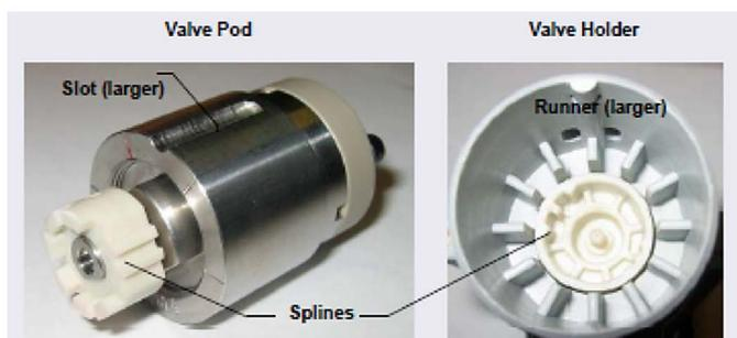
**Figure 4. Injection valve pod.**
