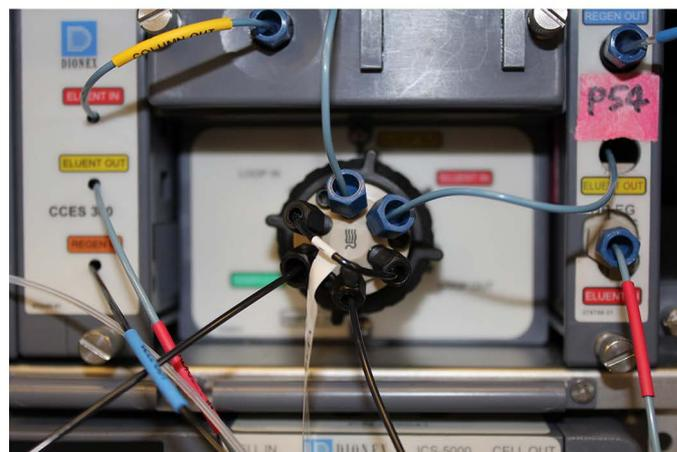
Figure 6. Dionex IonSwift concentrator column installed in ports 1 (top) and 4 (bottom) in the Dionex IC Cube 6-port valve.
