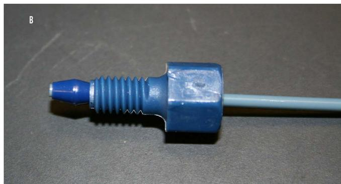
**Figure 3. A) Correct and B) incorrect placement of blue connector and ferrule on precision-cut tubing.**
