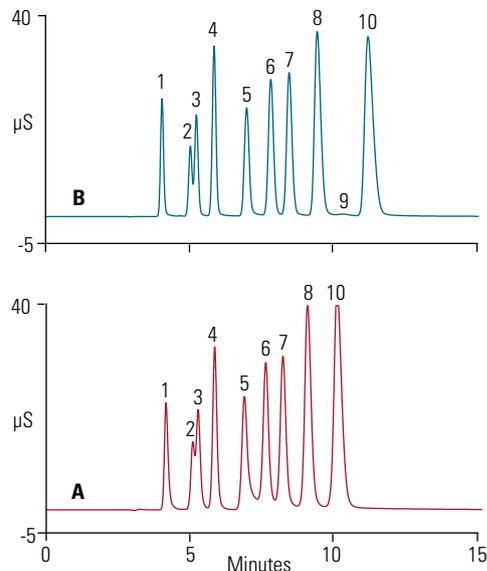
Figure 7. Comparison of the same anion standard simultaneously injected on A) 2 mm microbore and B) 0.4 mm capillary columns.
