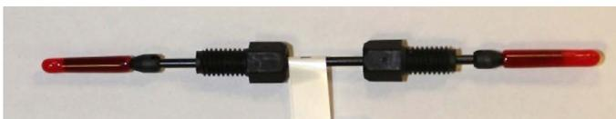
Figure 5. Dionex IonSwift concentrator column.
