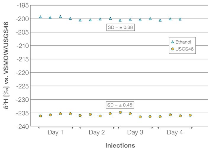
**Figure 4. Stability of hydrogen isotope delta value for two different samples over a period of 4 days.** Each data point is an average of 10 injections (N=10). The given standard deviation is related to the average values displayed.
