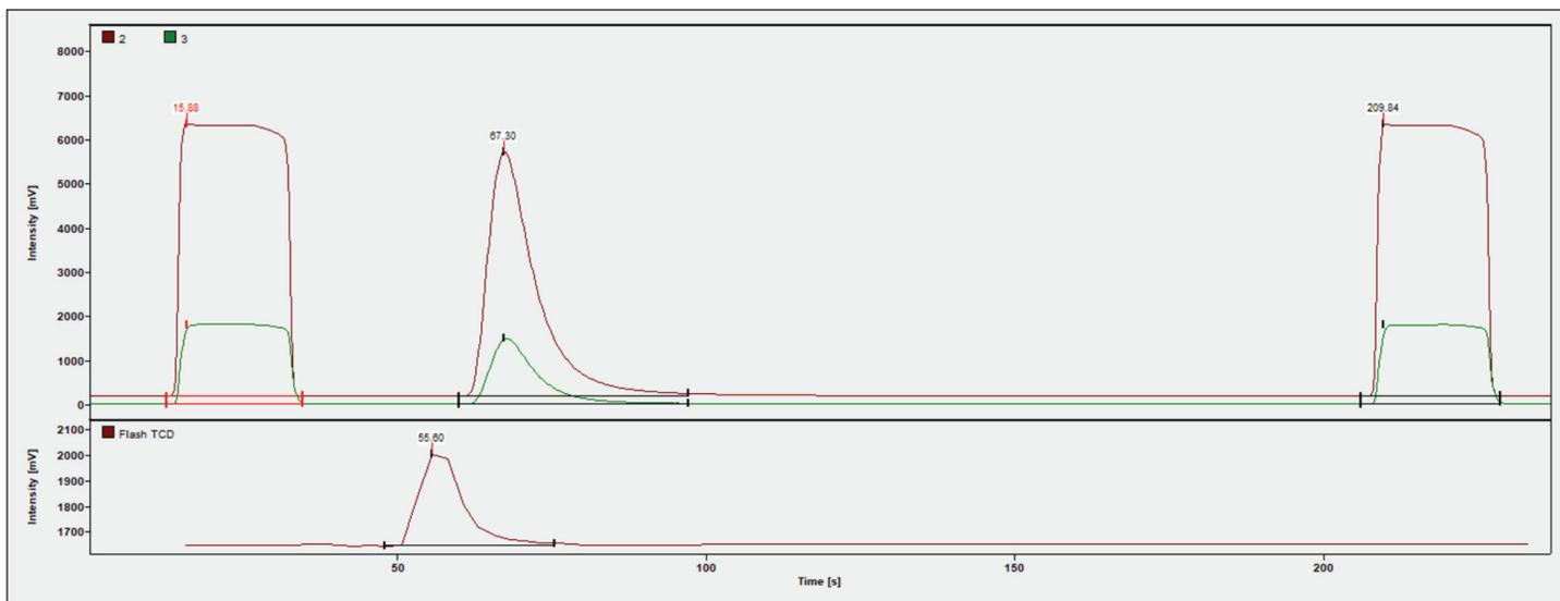
**Figure 2. Example chromatogram of 100 nL injection of USGS46 water standard.** Mass traces of  $m/z$  2 and 3 (above) as well as TCD trace (below) are shown. Squared pulses at the beginning and end of the chromatogram are reference gas injections. The second reference gas is not mandatory reducing the net analysis time to 110 s.
