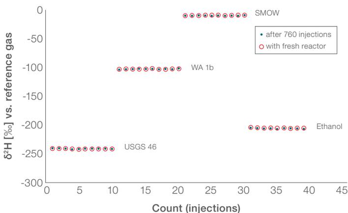
**Figure 3. Stability of analyses of four samples showing the hydrogen isotope data acquired at the beginning (red circles) and at the end of the long-term run (blue dots).**
