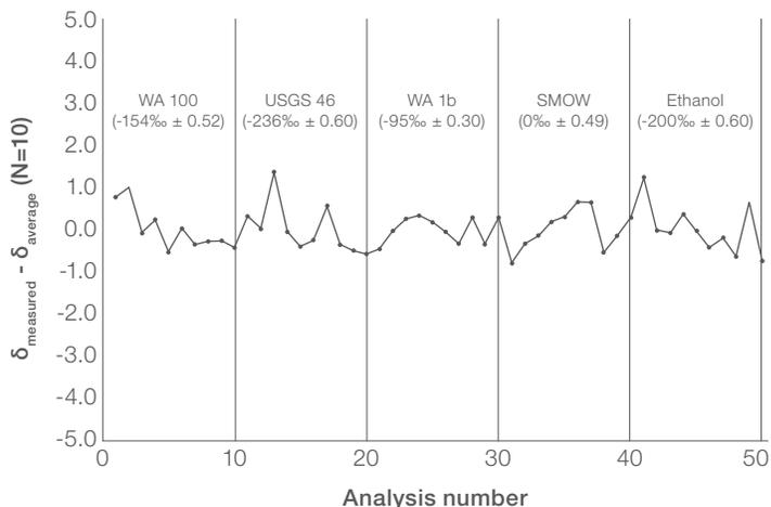
**Figure 1. Memory effects of a sequence of water analyses with 10 repetitions displayed as a difference between measured and the mean value of N=10 (data in brackets).**
