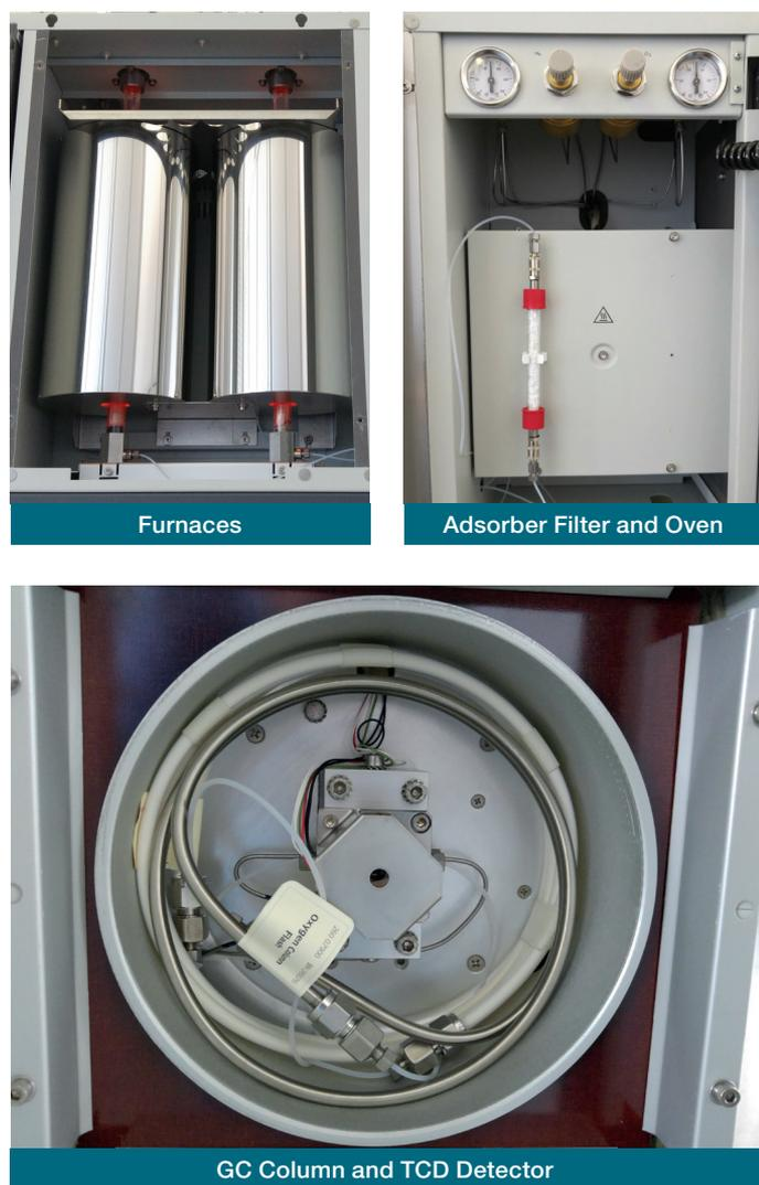
Figure 4. FlashSmart CHNS and oxygen internal circuits.
