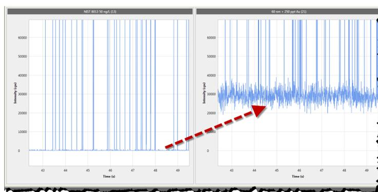
Figure 9. Comparison of background intensity for samples containing Au nanoparticles and 0 and  $0.25 \mu\text{g} \cdot \text{L}^{-1}$ .
