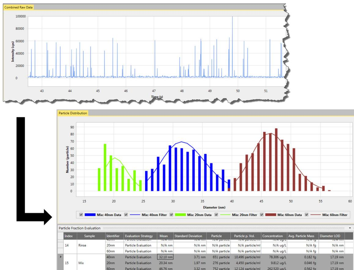
Figure 10. Statistical Data Evaluation available for each sample including estimation of dilution factor.
