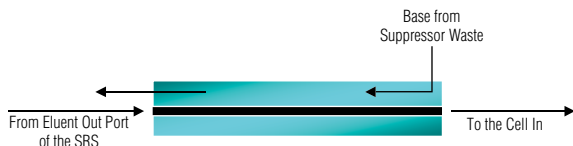
Figure 1. Carbonate removal device schematic.
