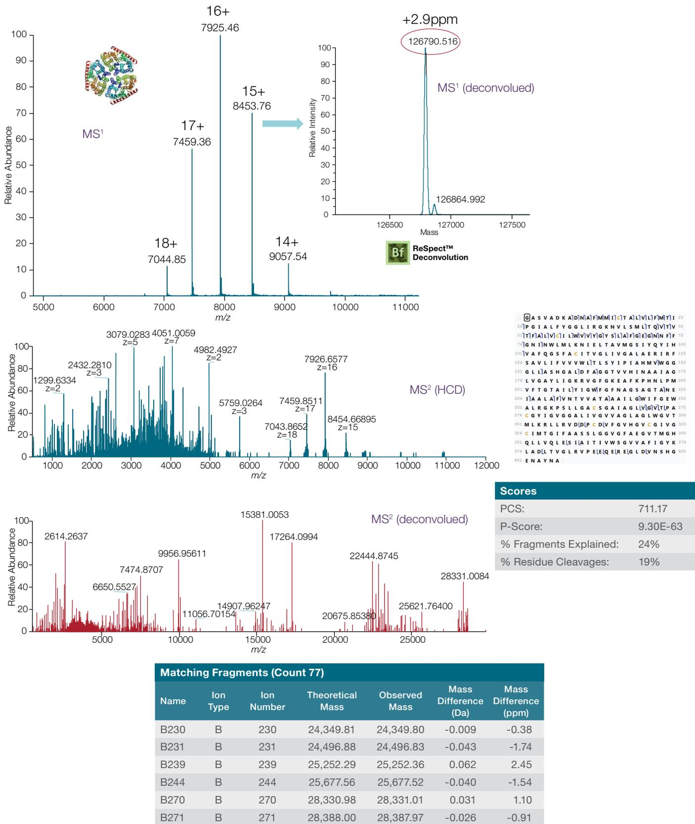
**Figure 6. Native MS and native top-down analysis of the AmtB membrane protein complex.** Low-ppm mass accuracy allowed confident identification of AmtB protein. Seventy-five b and y ions were identified, representing 19% residue cleavages.
