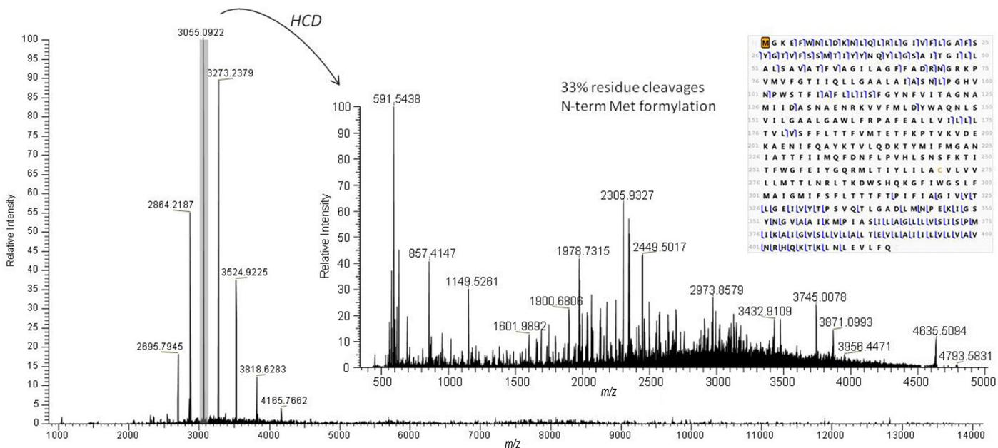
Figure 7. Native MS and native top-down analysis of the multidrug transporter membrane protein LmrP from *L. lactis* enabled identification of a total of 104 b and y ions, representing 33% residue cleavages
