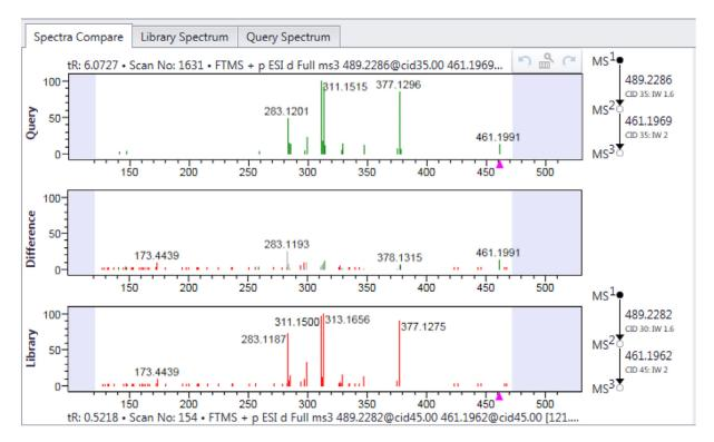
Figure 11. Spectral comparison of MS<sup>3</sup> at 461.1969 of component #1 vs MS<sup>3</sup> at 461.1962 of homosidenafil library compound
