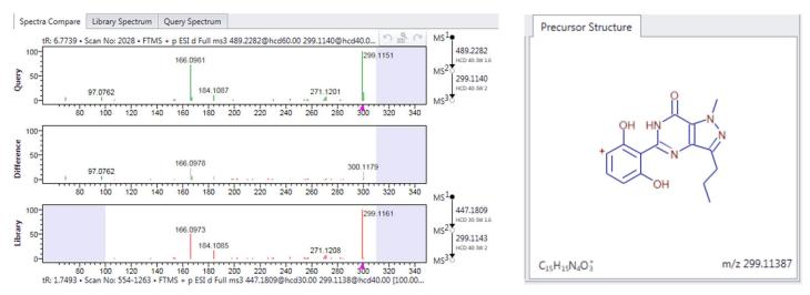
Figure 15. Example of substructure match on the MS<sup>3</sup> level, indicating the *m/z* 489 compounds (component #4 and #6) share this common substructure from the library
