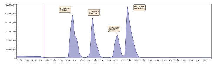
Figure 5. JCD detected four components with m/z of 489.2285, which corresponded to the four sildenafil compounds in the LC/MS mixture.
