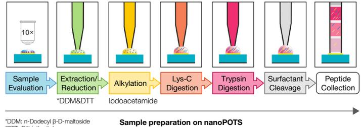
Figure 1. Protein digestion with nanoPOTS.
