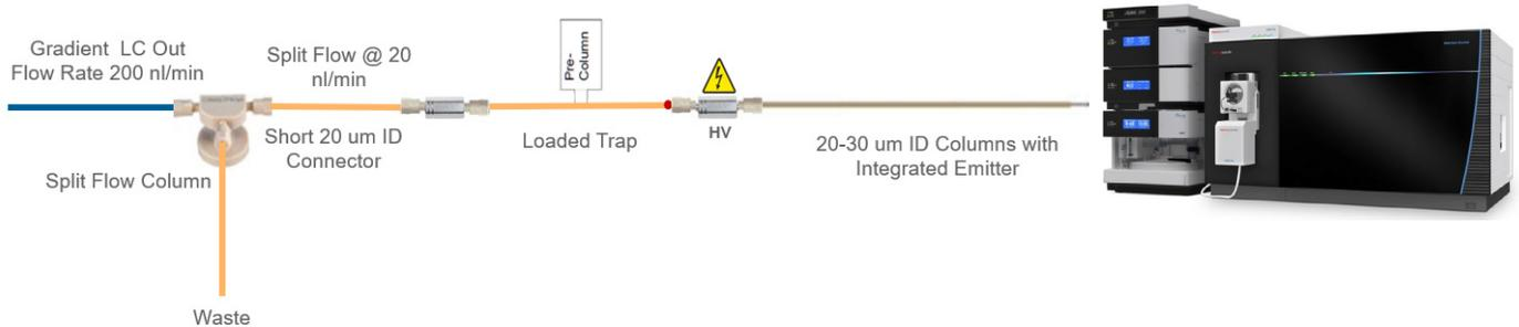
Figure 2. Ultra-sensitive low nanoflow LC-MS workflow for single-cell analysis.
