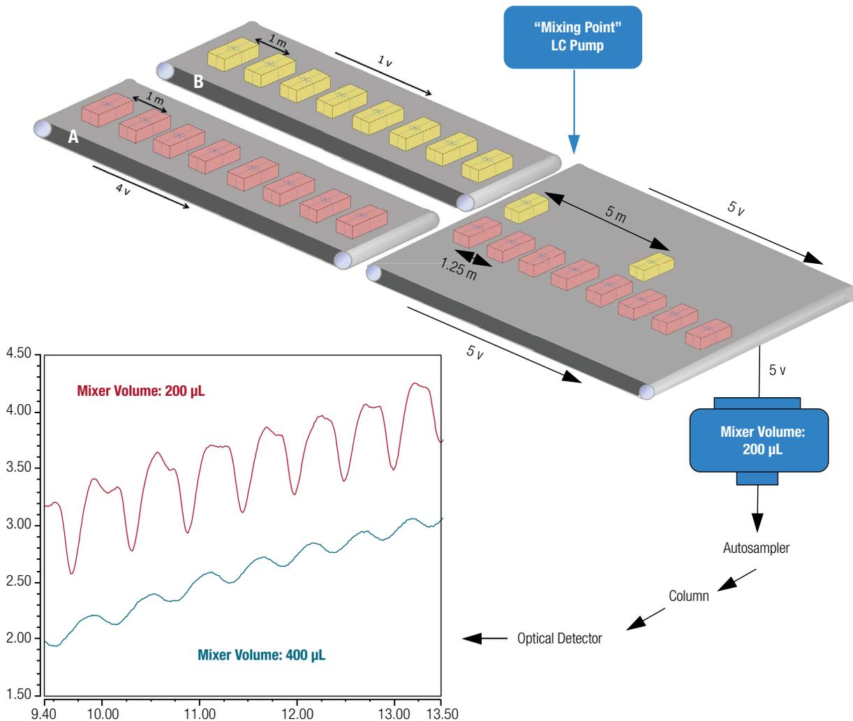
**Figure 3. The volume period of the LC pump.** (Top) Illustration of solvent flows A and B (represented as conveyor belts A and B) converging at the mixing point and a third conveyor belt to the mixer. The volume period of the LC pump is depicted as the space between parcels (e.g., 1 m) on the conveyor belts. (Bottom) Influence of the mixer size on baseline ripples at constant volume period using the UltiMate 3000 Binary RS system.
