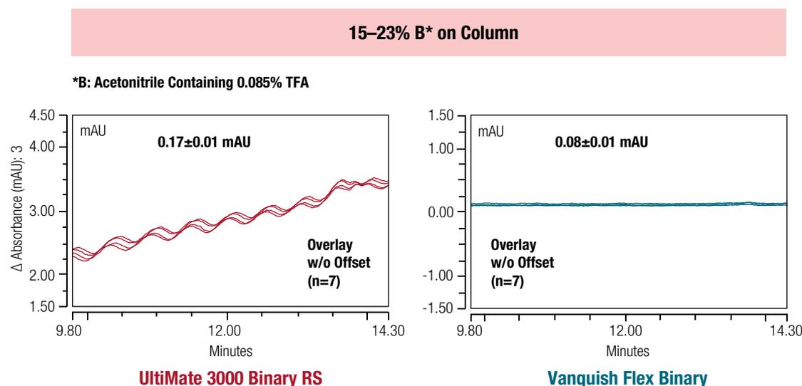
**Figure 6. System comparison of TFA mixing performance.** The UltiMate 3000 Binary RS system and the Vanquish Flex Binary system tested for TFA triggered mixing ripples with the same pump mixer volume (400  $\mu$ L) in a challenging TFA application (for details, see Figure 2).
