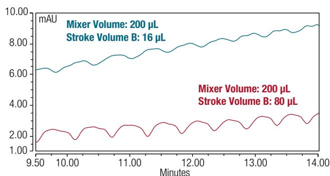
**Figure 5. Effect of small stroke volume.** (Top) Comparable GDVs between the UltiMate 3000 Binary RS system with 200  $\mu\text{L}$  mixer (red color) and with mimicked mixing point. (Bottom) Influence of small stroke volumes on TFA baseline ripples at fixed mixer volume (blue color).
