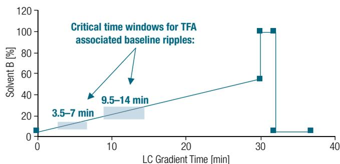
Figure 2. LC gradient with critical time windows for TFA associated baseline ripples highlighted.
