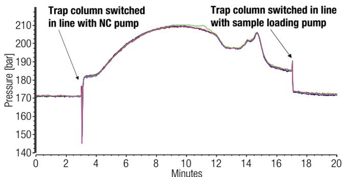
**Figure 3.** An overlay of five NC pump backpressure profiles corresponding to the analysis of 5 min (brown), 10 min (pink), 20 min (dark blue), and 45 min (black) antibody digests. The pressure profile for the analysis of the intact antibody is also shown for reference (turquoise).
