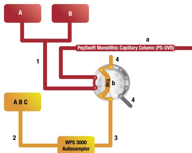
**Figure 1. Fluidic connections for pre-concentration of sample onto a monolithic column.** Note: The number and letter descriptions for each of the fluidic components are given in Table 1.
