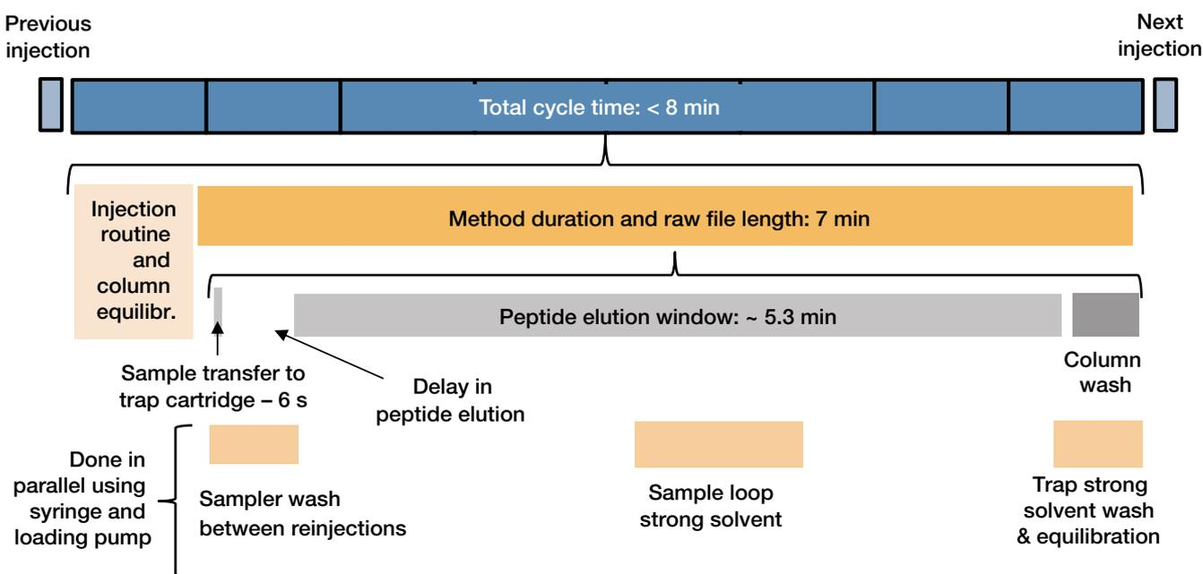
Figure 2. Schematic of the high-throughput low-flow LC-MS method
