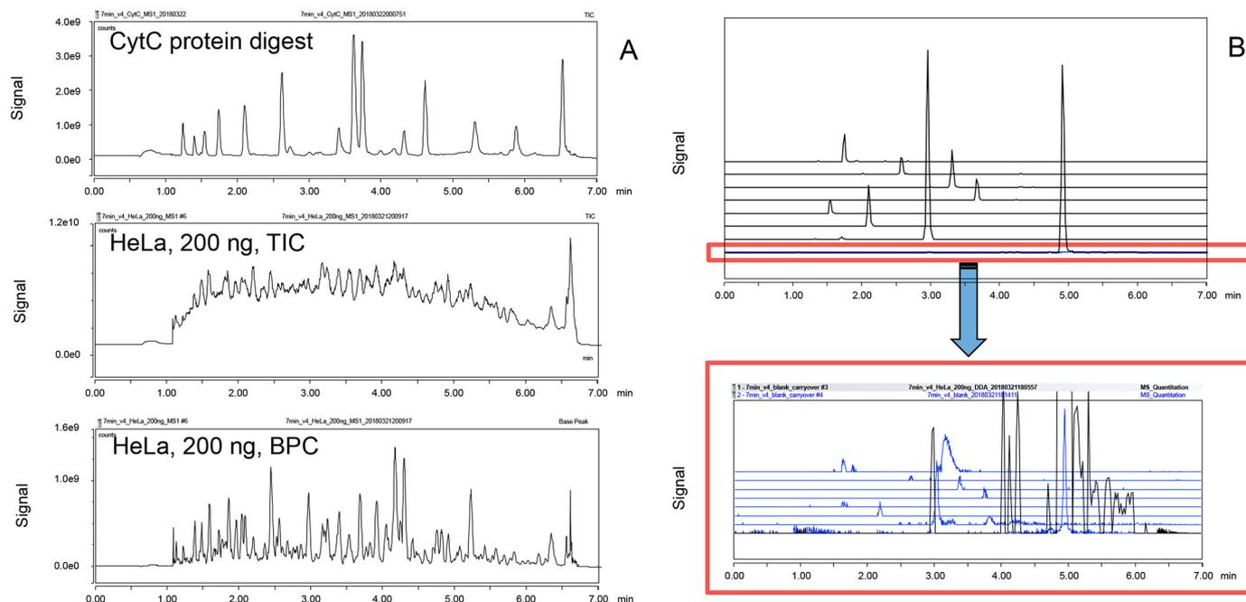
**Figure 3. Typical TIC and BPC profile of CytC and HeLa protein digests obtained using the high-throughput low-flow LC-MS method (A), and EICs of 200 ng HeLa peptide digest injections (black EIC traces) followed by blank injections (blue EIC traces) (B)**
