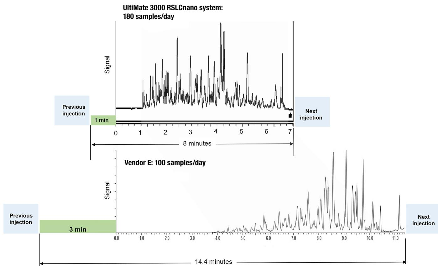
**Figure 5. Examples of base-peak chromatograms of HeLa cell lysate protein digest comparing the high-throughput LC method described in this work with a pre-defined 'locked' (non-editable) high-throughput method run using the LC system from vendor E**
