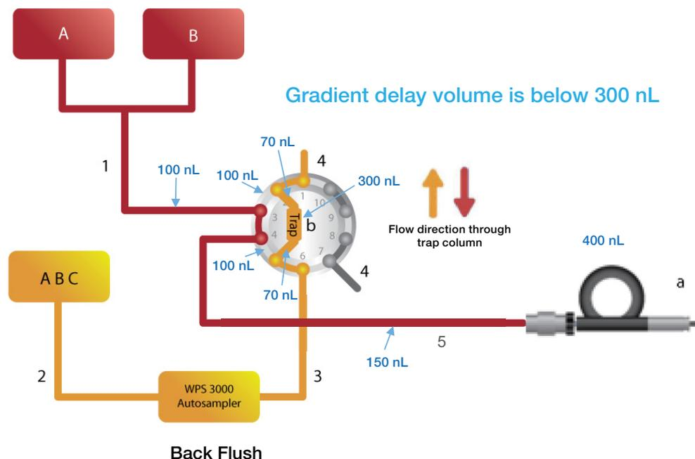
**Figure 1. Fluidic setup used for a pre-concentration of sample onto a nano column experiment.** Note: The number and letter descriptions for each of the fluidic components (in black) are given in Table 1. The values given in blue represent all the volumes from mixing of solvents A and B at the pump outlet until the emitter of the EASY-Spray column.
