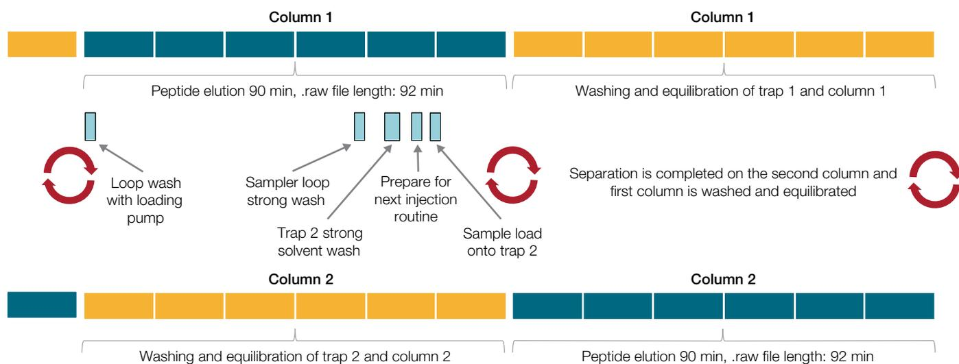
**Figure 5. Schematic of the pre-concentration tandem high-throughput low-flow LC method**
