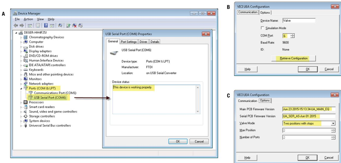
**Figure 4. Configuring the external VICI USB controller.** (A) The COM Port is displayed under the Device Manager of the Windows operating system. (B) The assigned COM port is selected in the Communication tab in the instrument configuration. (C) After retrieving the configuration, the Valve Mode is set to “Two positions with stops” in the Options tab.
