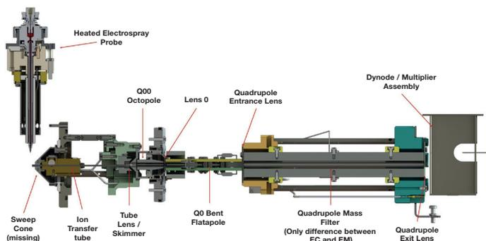
Figure 5. Schematic showing the components of the ion flow path.
