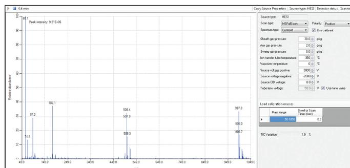
Figure 3. Real time scanning window with positive mode settings and spectrum.
