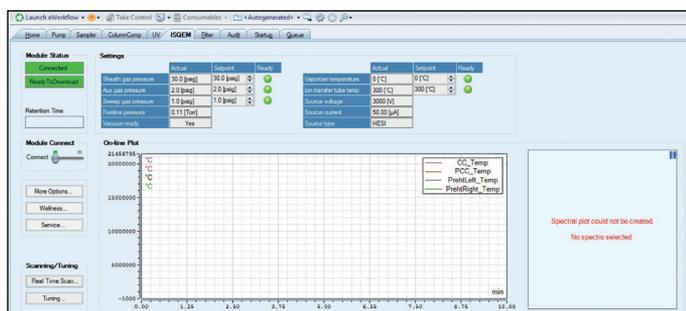
Figure 1. ISQ EC/EM ePanel.
