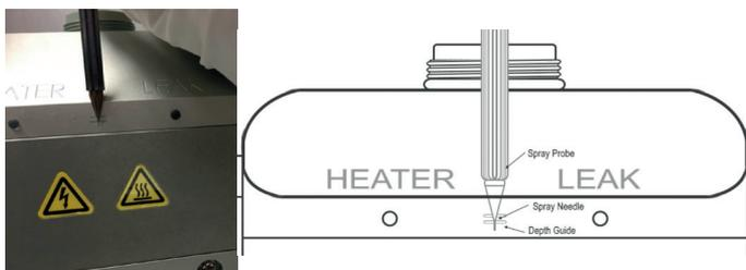
Figure 4. ESI capillary depth adjustment markings on the source housing.
