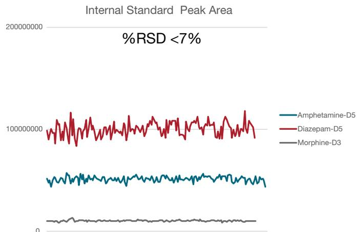
Figure 8. Robustness of peak area for over 400 injections for the internal standard, amphetamine-D5, diazepam-D5 and morphine-D3.
