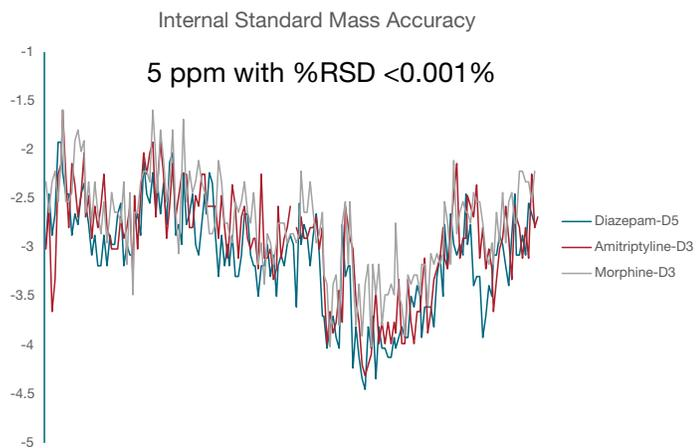
Figure 7. Robustness of mass accuracy over 400 injections for the internal standard, amphetamine-D5, diazepam-D5 and morphine-D3.
