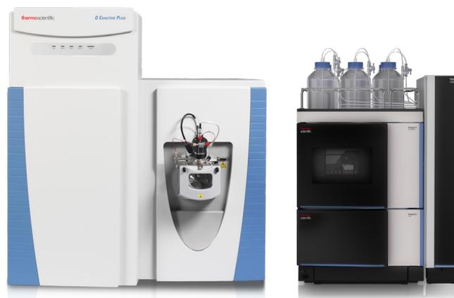
Figure 1. Q Exactive Plus MS coupled with Vanquish Flex UHPLC.
