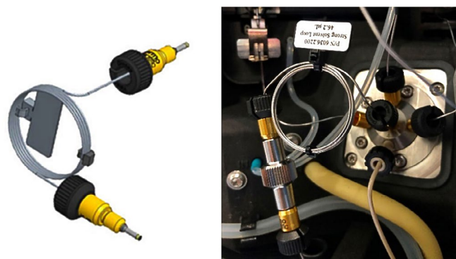
Figure 3. Schematic of the strong solvent loop on the left and installed on the instrument on the right
