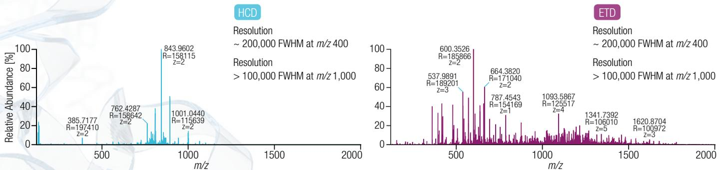
Analysis of histone H4 demonstrates the complementary nature of the HCD and ETD fragmentation techniques in the Orbitrap Elite instrument. Analysis using HCD and ETD in a single run significantly improved sequence coverage over each of the techniques used separately.
