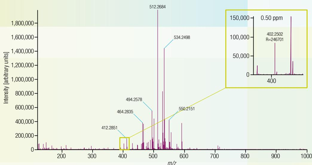
The Orbitrap Elite system provides accurate mass determination even in complex bile matrices. Here, an oxidative metabolite of buspirone eluting in the window of several bile matrix components was still detected with an absolute mass deviation of 0.5 ppm.
