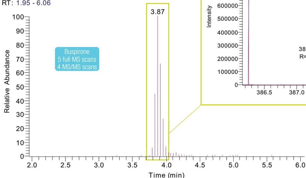
Even when acquiring MS and MS/MS data, the increased scan speed of the Orbitrap Elite system provides excellent coverage over narrow LC peaks. This analysis of buspirone demonstrates acquisition of full-scan data at a quarter of a million resolution at one Hz. In total, nine scans were acquired during the elution of the peak: five full MS scans and four MS/MS scans.
