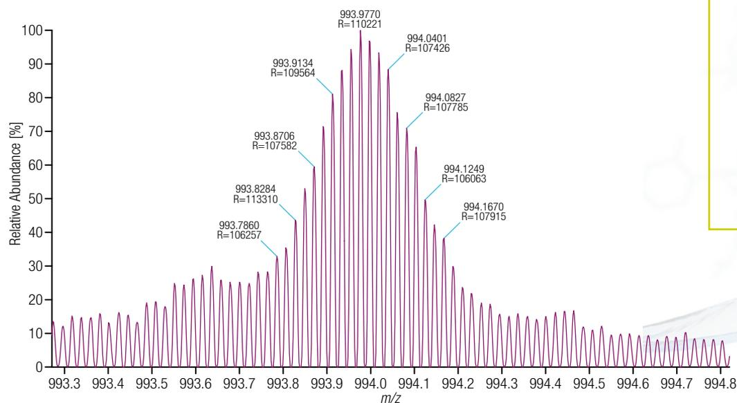
Analysis of intact yeast enolase (46.64 kDa) on the Orbitrap Elite hybrid MS demonstrates the superior resolution that makes it the new standard for proteomics applications.
