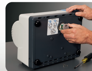
Infrared Source Replacement
