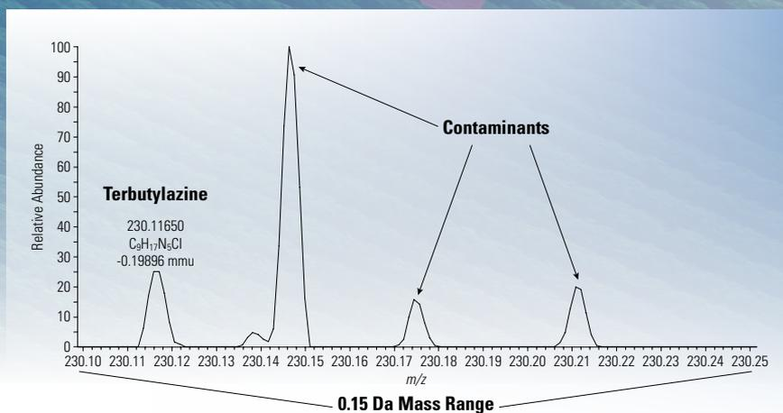
The high-resolution, accurate-mass capabilities of the Exactive Plus mass spectrometer make it ideally suited for nontargeted screening and quantitative experiments. The system provides full-scan data with mass resolution of up to 140,000 for structural confirmation, and mass accuracy to <1 ppm with internal calibration. Its high resolving power and mass accuracy enable accurate confirmation of all compounds, including isobaric pesticides.
