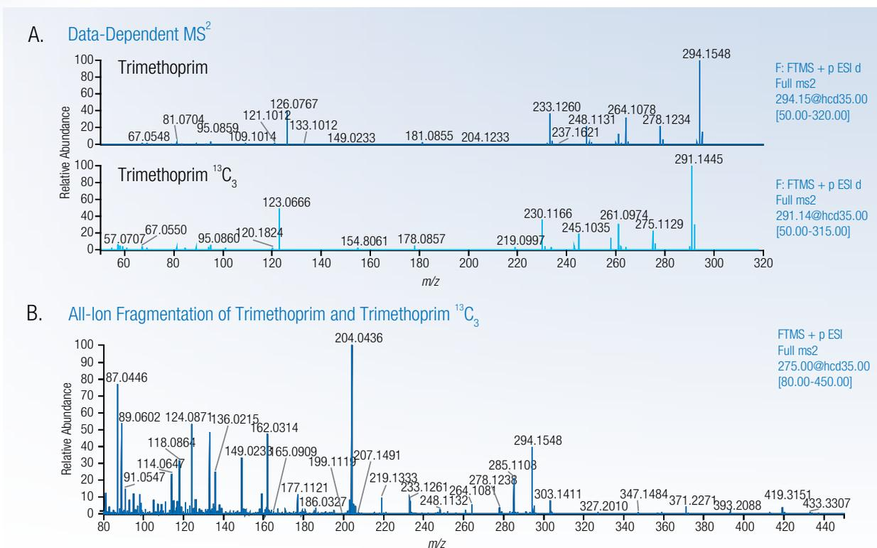
High-resolution data-dependent MS<sup>2</sup> on the Q Exactive MS easily distinguished a compound and its heavy-isotope-labeled internal standard (A) that could not be distinguished by all-ion fragmentation (B).
