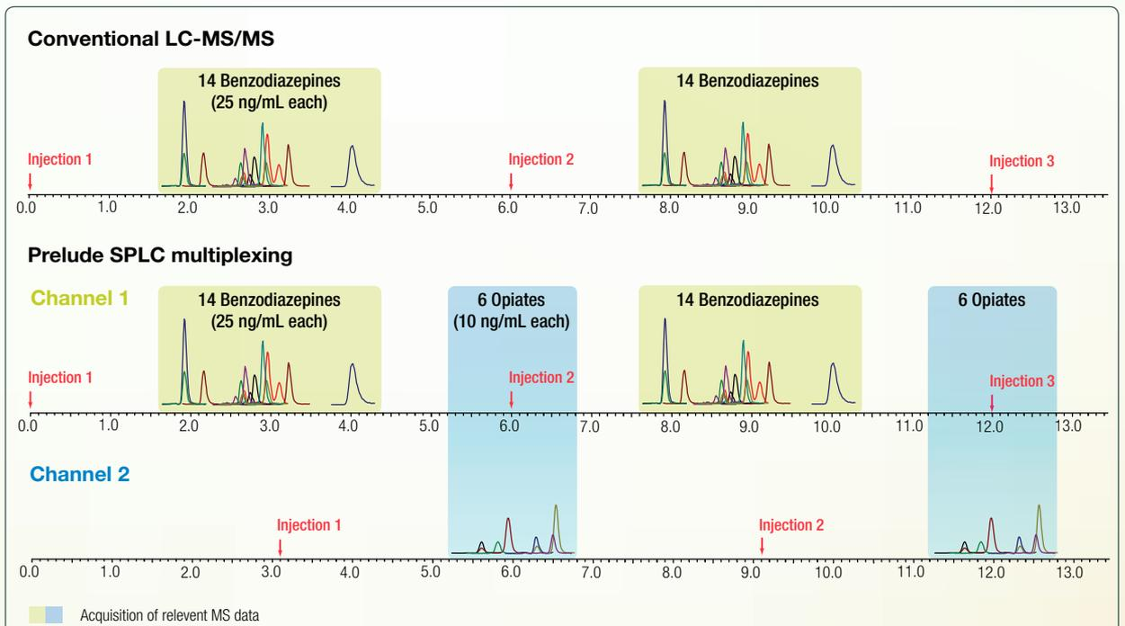
▲ Parallel analysis of 6 opiates (10 ng/mL) and 14 benzodiazepines (25 ng/mL) demonstrates how multiplexing on a Prelude SPLC can double productivity
