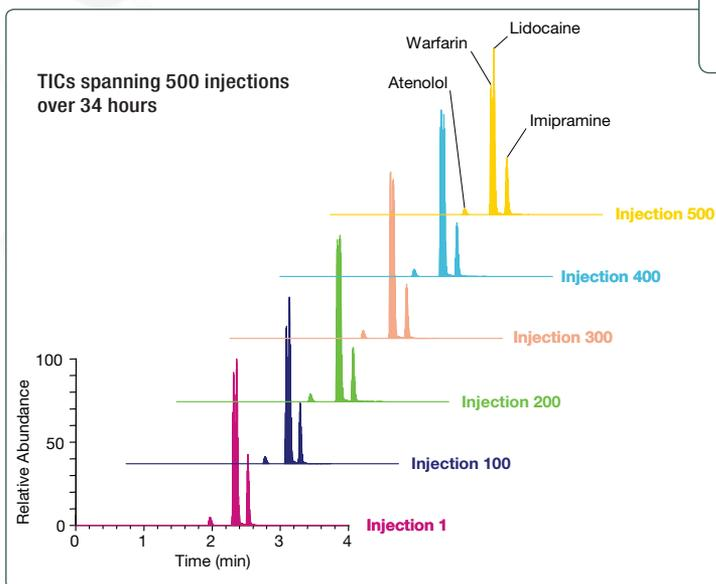
▲ 500 injections of four drugs in pooled, crashed human serum demonstrate the Prelude SPLC system's ability to generate reproducible separations in research and toxicology laboratories. Runs were multiplexed using the same TurboFlow and HPLC method on two chromatographic channels and a single mass spectrometer. MS area count RSDs for the 500 runs were <10% for all four compounds. No internal standard was used for normalization.
