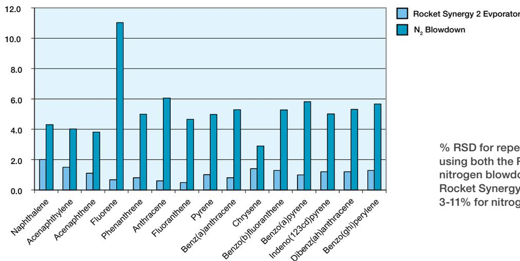
% RSD for repeat evaporations of PAH samples using both the Rocket Synergy 2 Evaporator and nitrogen blowdown. % RSD ranged from 1-2% for Rocket Synergy 2 Evaporator samples (n=6) and from 3-11% for nitrogen blowdown samples (n=6).
