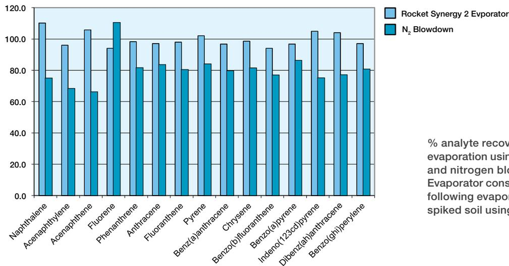
% analyte recovery for common PAHs following evaporation using both the Rocket Synergy 2 Evaporator and nitrogen blowdown (n = 6). The Rocket Synergy 2 Evaporator consistently generated higher % recoveries following evaporation. Extractions were performed from spiked soil using the Dionex ASE 350 system.
