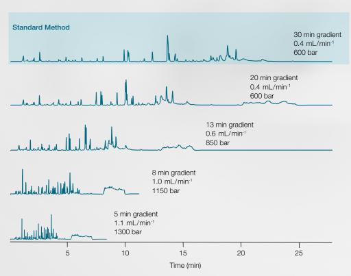
Accelerated peptide mapping utilizing the full power range of the Vanquish Horizon UHPLC system while maintaining 100% sequence coverage using a Thermo Scientific™ Acclaim™ RSLC 120, C18, 2.2 µm column.
