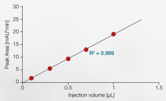
Autosampler linearity for even low injection volumes, here from 100 nL to 1  $\mu$ L.
