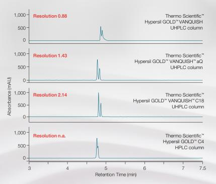
Automatic scouting of different column chemistries for fastest method development.
