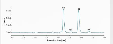
FLD chromatogram of the four aflatoxins: G2, G1, B2 and B1 at a concentration of 0.9  $\mu$ g/kg for G2 and B2 and 2.9  $\mu$ g/kg for G1 and B1.
