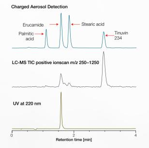
Unlike mass spectrometry and UV, the CAD is able to measure all analytes in the sample. Mass spectrometry (MS) requires the analyte to form gas phase ions while response by a UV detector depends upon the nature of the chromophore.
