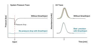
Significant reduction of pressure drop after injection using SmartInject Technology resulting in improved retention time reproducibility (6 replicates) and enhanced column lifetime.
