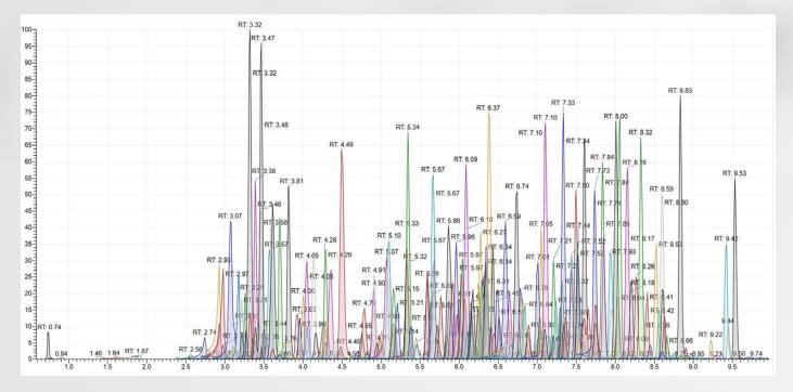
Extracted ion chromatogram of a matrix extracted spike (MES) of over 200 pesticide residues in baby food at 10 ng/g.
