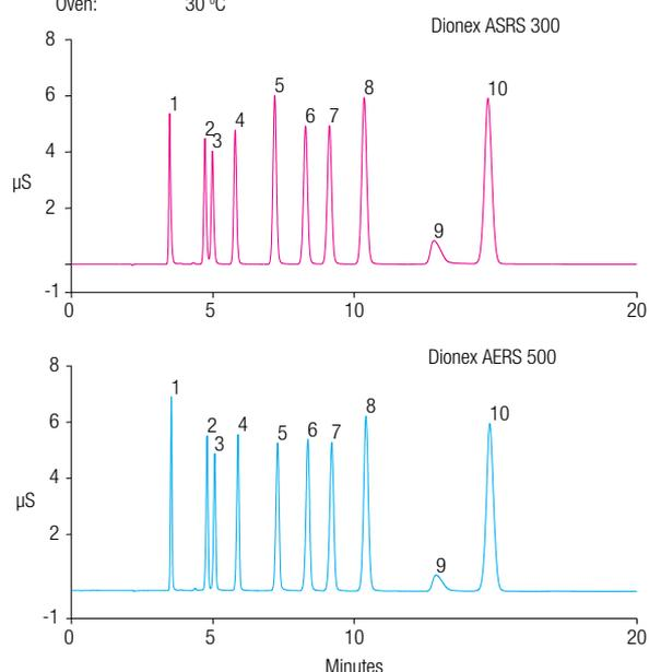
Figure 3: Comparison of the Dionex AERS 500 suppressor to the Dionex ASRS 300 suppressor using an inorganic anion standard. The Dionex AERS 500 suppressor outperforms the Dionex ASRS 300 suppressor, as shown by the peak efficiency and resolution
