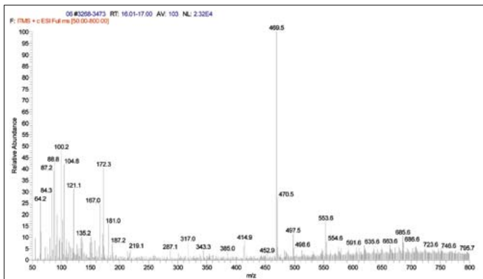
Fig. 13a-c. MS spectrum from 50 – 800 m/z in positive mode using LTQ Orbitrap XL. (a) Full MS scan of Vendor X methanol at end of gradient. (b) Full MS scan of Fisher Chemical Optima methanol (A456). (c) Full MS scan of Vendor B methanol.
