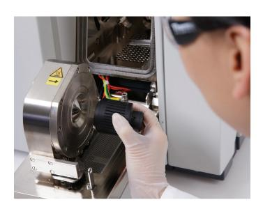
The Thermo Scientific™ iCAP™ Qnova™ Series ICP-MS features a unique interface designed to simplify user maintenance and allow for customization to ensure maximum performance based on the sample type.
