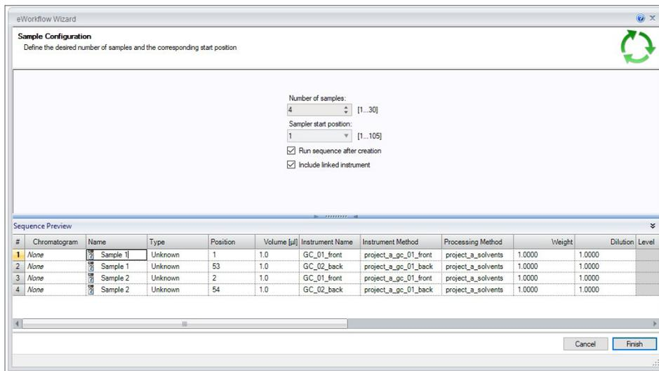
You can create a sequence using either one or both linked instruments by simply selecting the 'include linked instrument' option. The eWorkflow Wizard shows the instrument name as part of the sequence preview, the autosampler rack preview, however, is disabled when linked instruments are used
