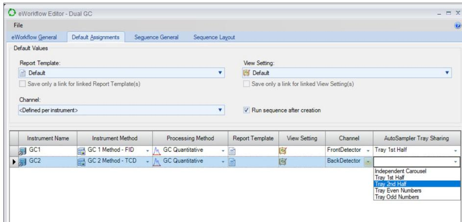
**Default Assignments in the eWorkflow Editor ensure correct method, report and channel selection for each instrument. Where instruments are linked, the autosampler tray sharing can be defined**
