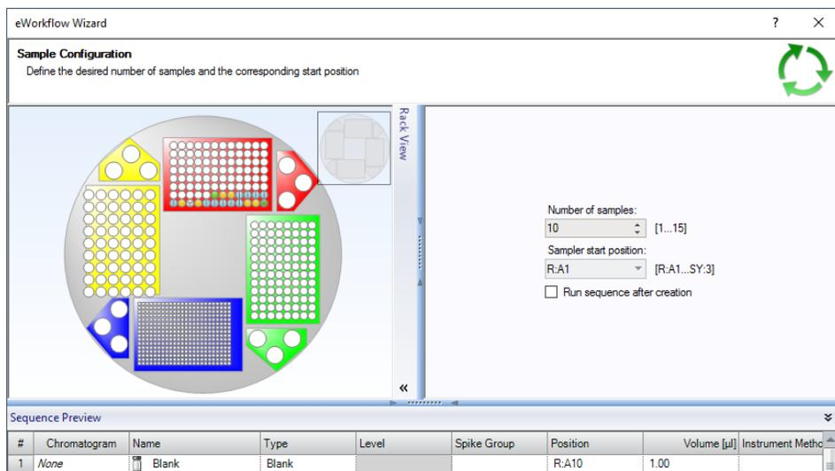
**The eWorkflow Wizard shows a sequence and autosampler rack preview with easy selection of the number and positions of samples. Edits are also possible in this window, if enabled**
