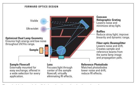
$\label{thm:continuous} The \ optical \ design \ maximizes \ light \ throughput \ improving \ signal-to-noise \ ratios.$
