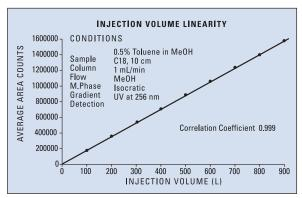
Injection linearity is unsurpassed from 1  $\mu L$  to over 1000  $\mu L$  with highly-controlled injection processes and accurate syringe drives.
