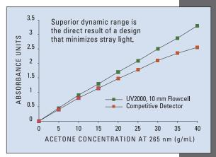
Absorbance non-linearity is less than 5% at up to  $2.0~\mathrm{AU}$  at  $254~\mathrm{nm}$ .
