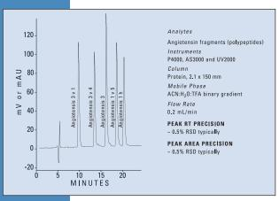
Peak shape, peak area and retention time precision are excellent with the P4000 solvent system.
