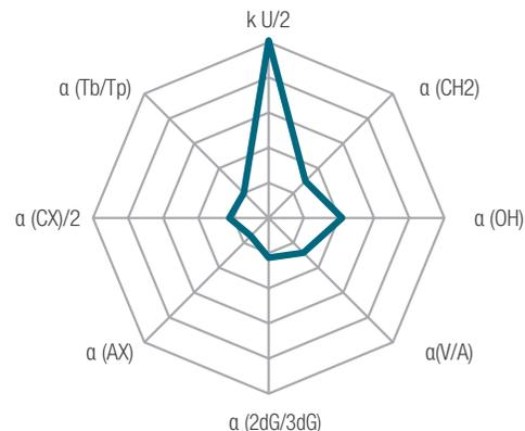
The zwitterionic material offers the highest absolute retention and good hydrophobic, hydrophilic and isomeric selectivity. Low ion-exchange properties are demonstrated by this neutral material.
