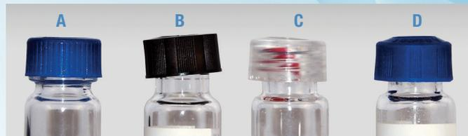
Examples of vial and closure misalignment/deformation. (A) SureStop vial self-aligning cap; (B) generic vial, cap tilt; (C) generic vial, septum dislodged; and (D) generic vial, deformed top.
