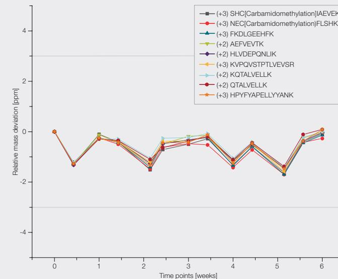
**Stable mass accuracy** on Orbitrap Exploris MX mass detectors: <3 ppm mass deviation **over 6 weeks** with one-point calibration.
