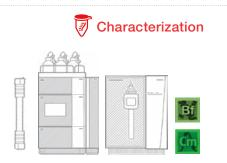
**Vanquish UHPLC-Orbitrap Exploris 240 MS** Using the high-resolution accurate mass and data, one can confidently identify, map, and relatively quantitate oligonucleotides, impurities, and degradation products in a single experiment
