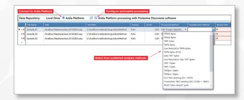
To set up the automation process, users have the simple task of indicating before submitting an acquisition request to publish the data to the Ardia Platform and choose the methods to use for data processing within Proteome Discoverer software.
