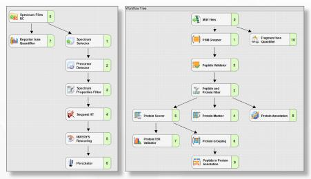
Spectra are streamed from the top of the workflow and pass through nodes that perform filtering, peptide ID, quantification, FDR calculation, grouping, and more.
