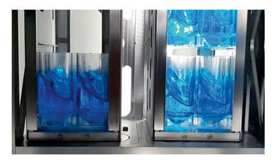
The Cytomat 2 Selector Automated Shaking Incubator uses consistent true orbital shaking patterns for reproducible results
