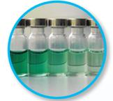
Calibration dilution with internal standard
