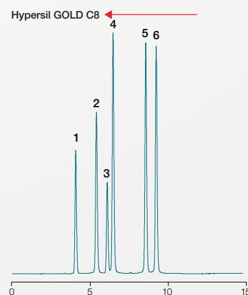
When analyzed using a Thermo Scientific™ Hypersil GOLD™ aQ HPLC column, the chromatogram below shows that the same elution order as the Hypersil GOLD column results. There is extra retention of analytes 2 and 4, which can be attributed to the fact that the gallocatechins have an additional OH group to interact with the polar endcapping.
