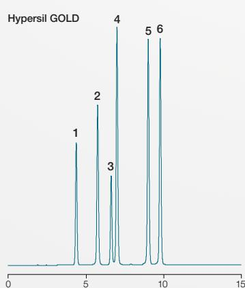
When analyzed using a Thermo Scientific™ Hypersil GOLD™ C8 column, as shown below, all six analytes maintain the same elution order, but with reduced retention, which is to be expected as hydrophobic interactions are reduced.
