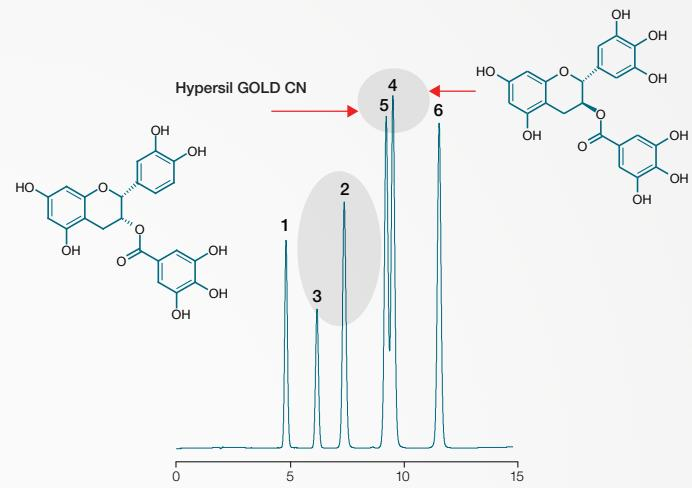
The chromatogram below shows the retention of catechins using Thermo Scientific™ Hypersil GOLD™ Phenyl HPLC columns.
